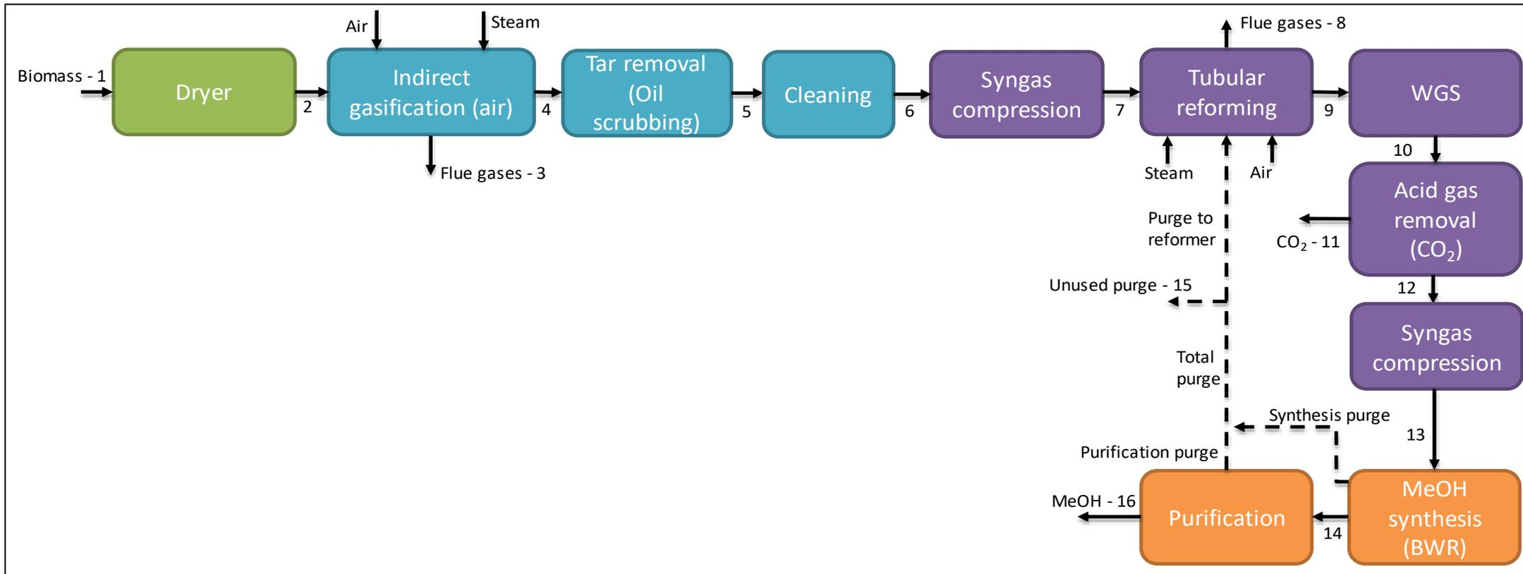
Figure 2. Simplified process flow-sheet of the Base Case
