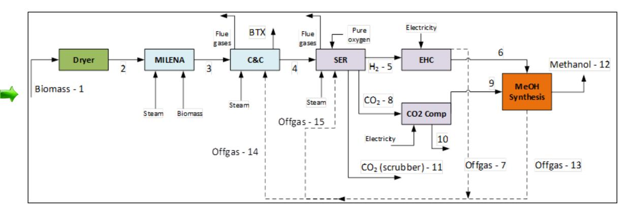
**Figure 3.** Simplified process flow-sheet of the CONVERGE Case
