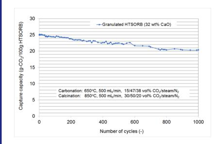
Long-term sorption capacity: stabilized at < 20 g-CO<sub>2</sub>/100g sorbent after 1000 carbonation-calcination cycles
